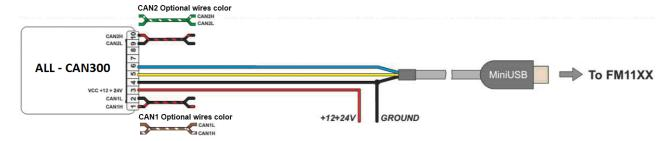
Figure 54 ALL-CAN300 Adapter connection cable pinout
