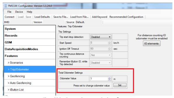
Figure 36 Continuous odometer setting in configurator.
