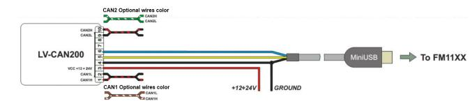
Figure 53 LV-CAN200 Adapter connection cable pinout
