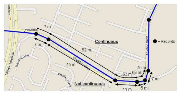
Figure 33 Trip continuous distance counting parameter example
