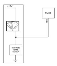
Figure 10 Fuel sensor scheme
