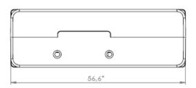
Figure 1 FMA120 view & dimensions (tolerance ±2mm)
