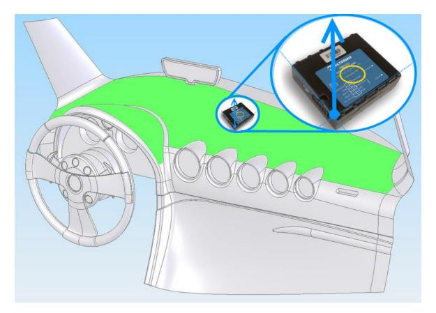
Figure 51 Correct placement of FMA120
