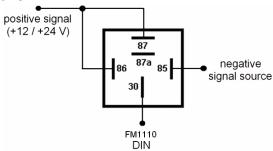
Figure 12 Inverting relay connection
