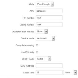
Using Passthrough Mode will disable most of the router capabilities!
