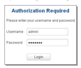
Enter the default password, which is "admin01" into the "Password" field and then either click Login with your mouse or press the Enter key. You have now successfully logged into the RUT850!
