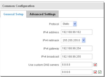
This is the configuration setup for when you select the static protocol.
