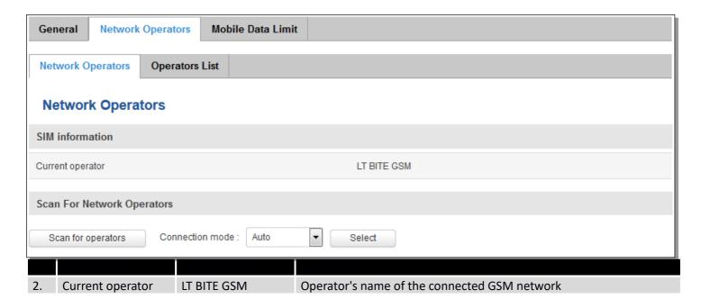
Note: after clicking Scan for operators' button- You will lose current mobile connection! For changing network operator status have to be available. There is manual connection to network operator, you have to fill numeric name, and it's have to be available.
