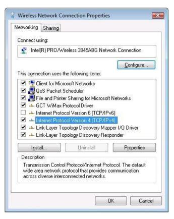
6. By default the router is going to have DHCP enabled, which means that if you select "Obtain an IP address automatically" and "Obtain DNS server address automatically", the router should lease you an IP and you should be ready to login.
