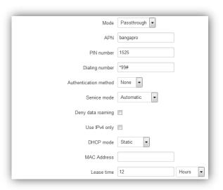
Using Passthrough Mode will disable most of the router capabilities!
