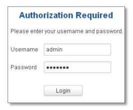
Enter the default password, which is "admin01" into the "Password" field and then either click Login with your mouse or press the Enter key. You have now successfully logged into the RUT950!
