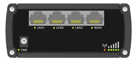
RUT9xx can be powered from power socket and over Ethernet simultaneously. Power socket has higher priority meaning that the device will draw power from power socket as long as it is available.
